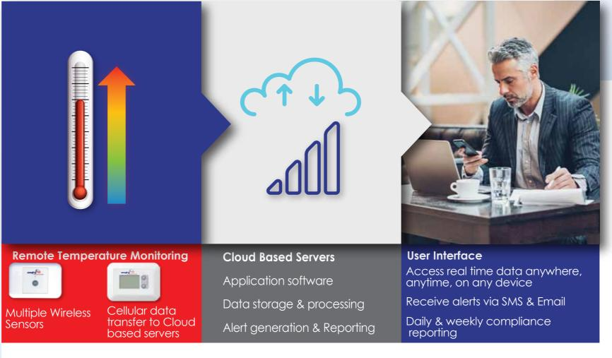
The Sentry Temperature Monitoring System independently monitors temperatures against set points and provides alerts when the set points are breached.
